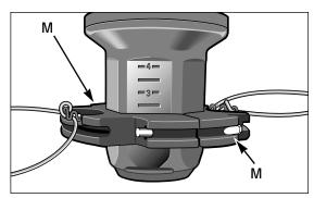
Figure 2-4: Check trimmer head hardware for tightness.
